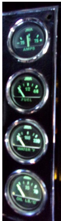
Center Console Gauges Illuminated With Hybrid Green LEDs
